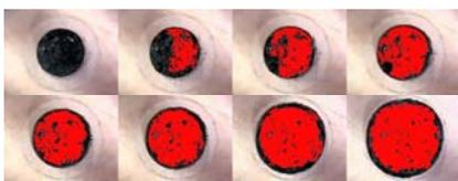
**Fig. 1b:** Visualization of effective electrode area with increasing pressure. One objective of the project is to reduce to a minimum the mechanical deformation energy to a minimum which is required to increase the effective electrode area to a maximum, thus increasing the efficiency of mechanical to electrical conversion.
